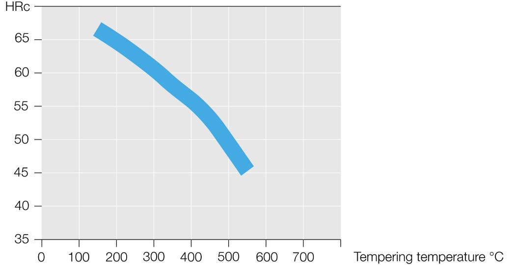
If your harden in oil, we recommend to not pass over the annealing temperature of 820°C to avoid cracks. The water should be pre-heated at about 50°C. The above curves indicate the results of determinate section of a curtain size of 5 mm. The result after heat treatment can be slightly different than shown on this curve, depending on the shape and size of the part.
