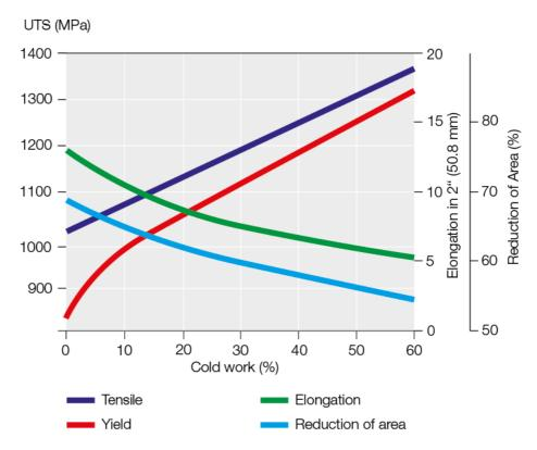
A plastic deformation made before aging, permits to reach still higher mechanical properties. A heavy cold deformation like for springs (Condition C) permits to reduce the duration of a 455°C aging to 30 minutes.
